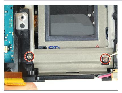
• Remove two 6 mm J000 screws from the left of the shutter.
