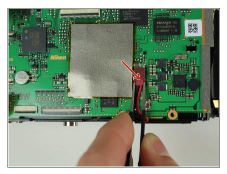
Carefully disconnect the red connector with tweezers.
