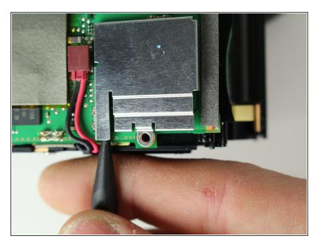
Gently lift the right motherboard shield off with the tip of a spudger.
