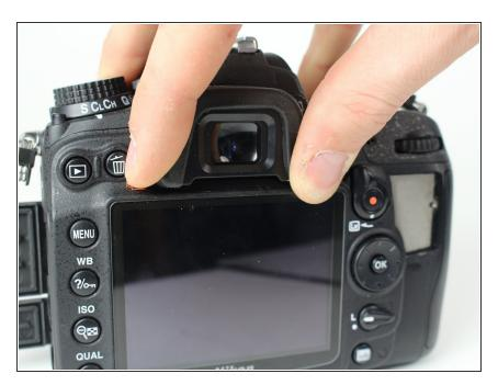
Pull the eyepiece cover up to remove it.
