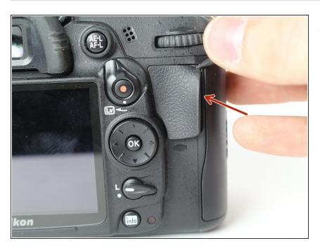
Peel the rear rubber piece off with tweezers.
