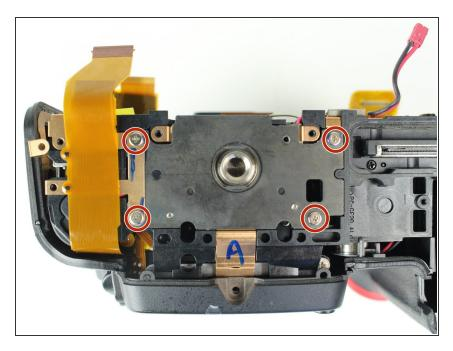
Remove four 6 mm J000 screws securing the tripod plate.
