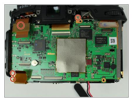
Remove four 3.5 mm J000 screws securing the motherboard.
