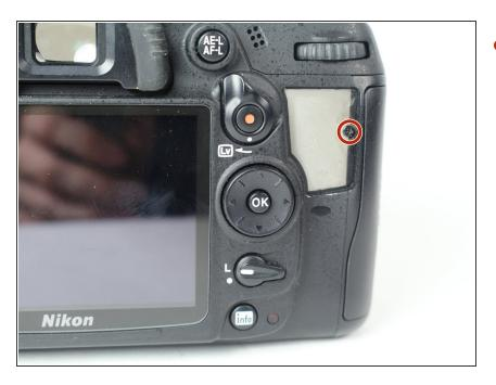
Remove one 4.25 mm J000 screw from behind the rear rubber piece.
