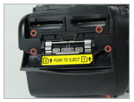
Remove four 6 mm J000 screws that secure the SD card cover.
