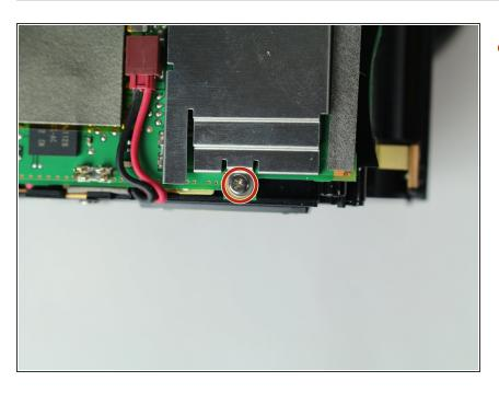
Remove one 3.5 mm J000 screw securing the right motherboard shield.
