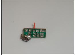
All that is left of a 3xAA battery pack and switch following the removal of corroded batteries.
