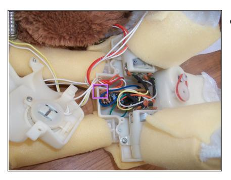
Spaghetti junction! The motherboard is sitting vertically inside the box. To lever it out use a flathead screwdriver between the uppermost board edge and the plastic casing. (marked on photo in pink) Push the screwdriver so that the edge of board lifts and you are able to grab with your fingers.
