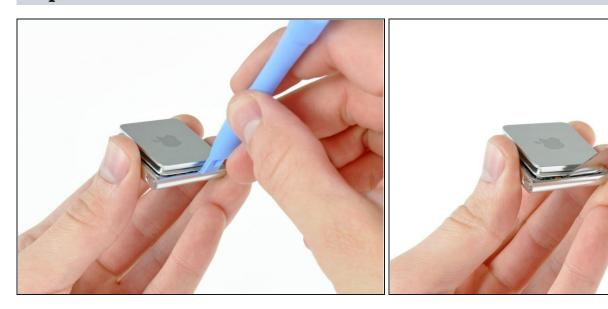
• Use a combination of iPod opening tools and metal spudgers to pry the rear panel away from the Shuffle by the seam nearest the ON/OFF switch.
