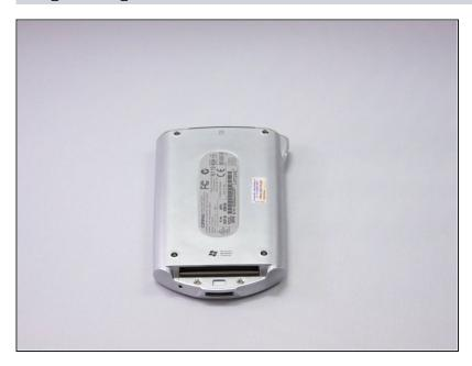
To start the disassembly of iPAQ speaker shown by picture, you must place speaker on a flat surface with the screen laying down.
