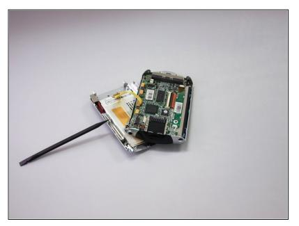
You must carefully remove the back cover using a plastic opening tool against the grooves along the sides of the iPAQ speaker.
