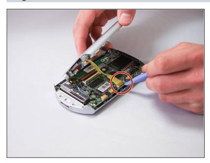
Using the plastic opening tool, carefully detach the yellow ribbon from the connector pins to separate the iPAQ speaker into two halves. (This step isn't necessary for speaker removal it will just make the process a lot easier.)
