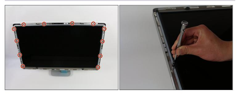
• Unscrew the 12 screws around the side edges and the top of the LCD with the TR 10 Screwdriver.
