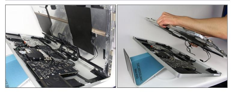
• The LCD has now been fully disconnected from the casing and can be repaired/replaced!
