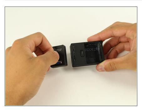
Use the battery tab to pull the battery out of the device.
