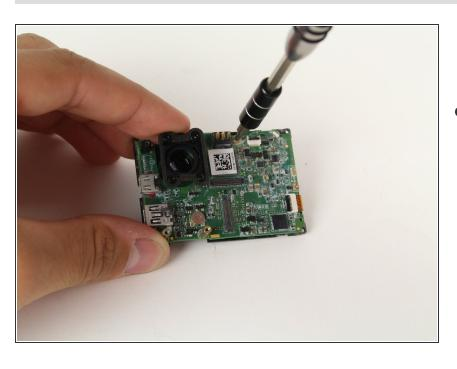
Using your trusty screwdriver, remove the single 3.2mm PH00 screw connecting the motherboard to the midframe.
