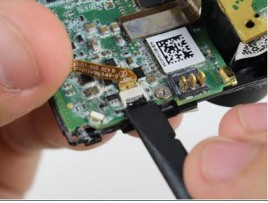
Remove the ribbon cable connecting the housing to the motherboard by flicking up the black clip with the spudger tool and gently pulling the cable out.
