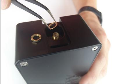
• Remove the nut and washer from the RF connector, located where the antenna was connected.
