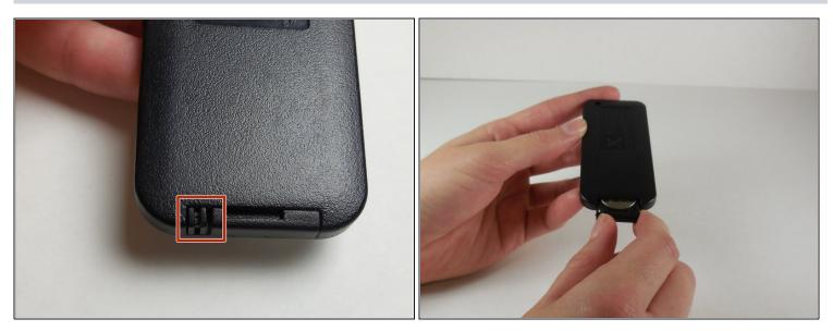
• Open battery tray by pushing right on the boxed tab and pulling the battery tray out.
