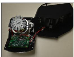
Using the Phillips #2 screwdriver, remove these six screws (13mm long, 6mm head diameter).
