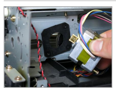
Remove the stepper motor by pulling it straight out.
