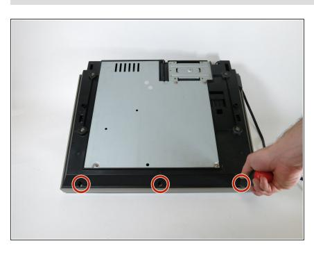
Remove the three 19 mm screws located in the recessed holes on the edge of the black underside panel using a Phillips #2 screwdriver.
