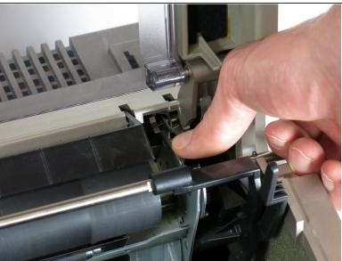
Unlock the roller wheel by simultaneously pressing down on the two spring levers on the left and right of the roller ends.
