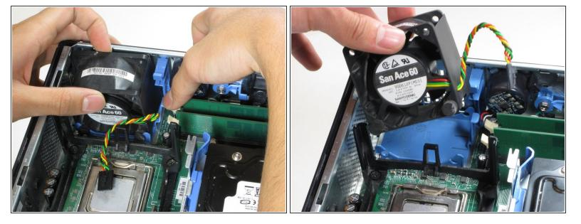
Press on the blue release tab and pull the upper fan out of the computer.
