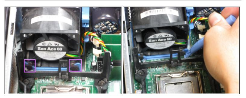
Remove the rubber grommets from the base of the fan. A spudger may be useful.
