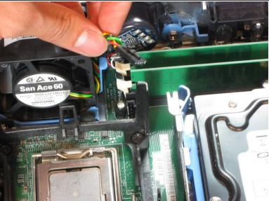
Remove the power supply that connects the upper fan to the motherboard. The power supply has black, red, green and yellow wires.
