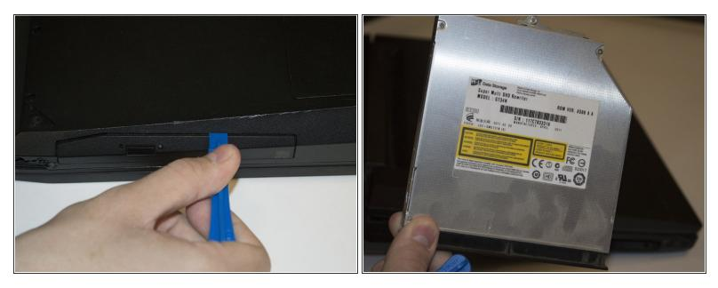
• Lastly, use a plastic opening tool to remove the optical drive from its slot.
