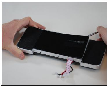
• Using the metal spudger, gently lift the face plate away from the display.
