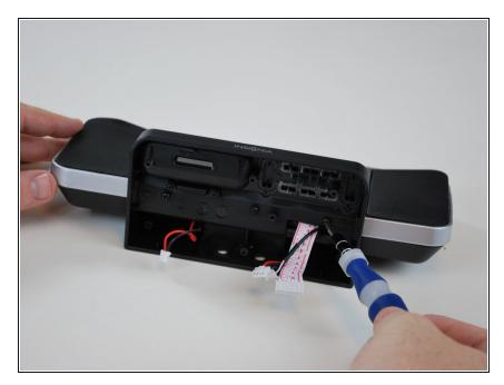
Using the Phillips screwdriver, remove the three screws that run along the center of the base.
