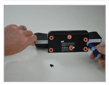
Use a Phillips screwdriver to remove the six 11 mm screws on the bottom of the device.
