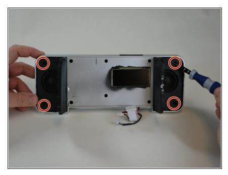
Using the Phillips screwdriver, remove the four screws shown here.
