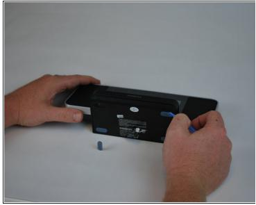
• Using a plastic opening tool, peel off the adhesive gel stoppers.
