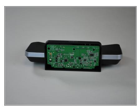
Remove the bottom cover from the device to reveal the motherboard.
