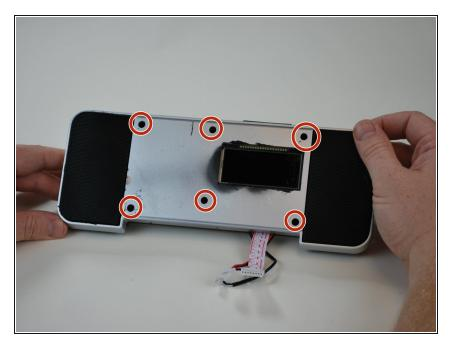
Once the face plate is removed, use the Phillips screwdriver to remove the six screws shown here.
