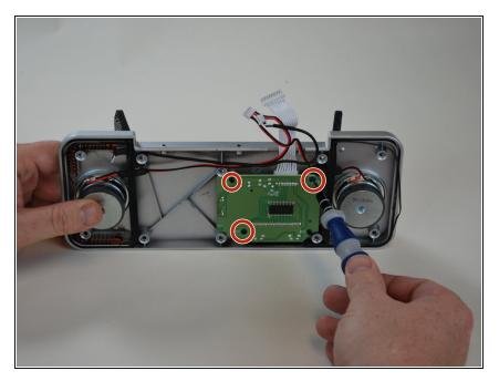
Using the Phillips screwdriver, remove the three screws shown here.
