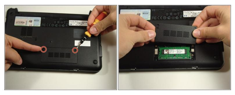
Use a Philips #0 screwdriver to unscrew the two screws covering the memory compartment on the bottom of the laptop and remove the cover.
