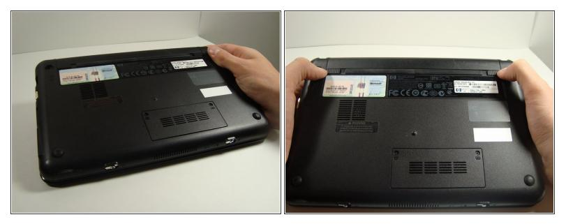
Locate the battery and the battery tabs on the bottom of the Compaq Mini.
