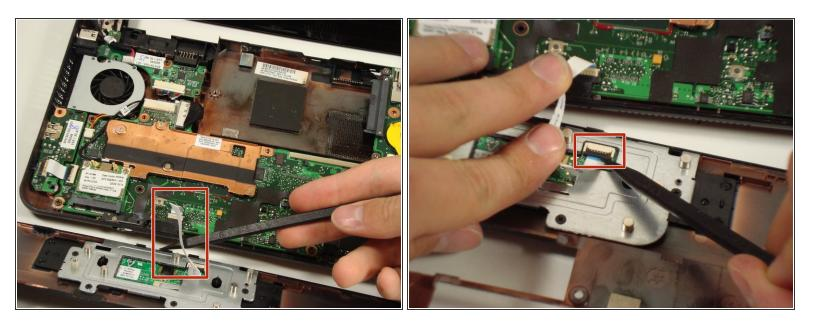
• Remove the cable by carefully pulling it up.
