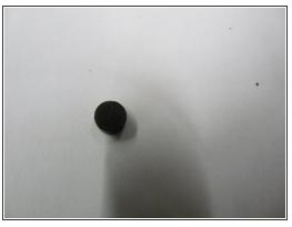
On the ear bud you will see a magnet on the inside of the black encasing, Remove the Magnet from the encasing.
