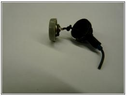
Take the silver covering off of the ear bud, notice the black wire connecting the two (the wire should be knotted)
