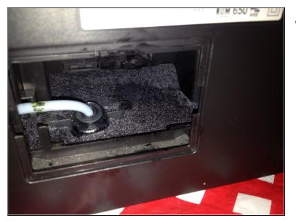
As you can see, the pad is full with waste ink and is larger than the small door that gives you access to it, meaning it is not meant to be changed by mortals.
