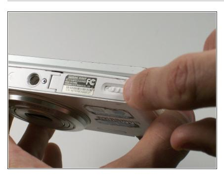
Slide the lock towards the middle of the camera, in the same direction of the arrow.
