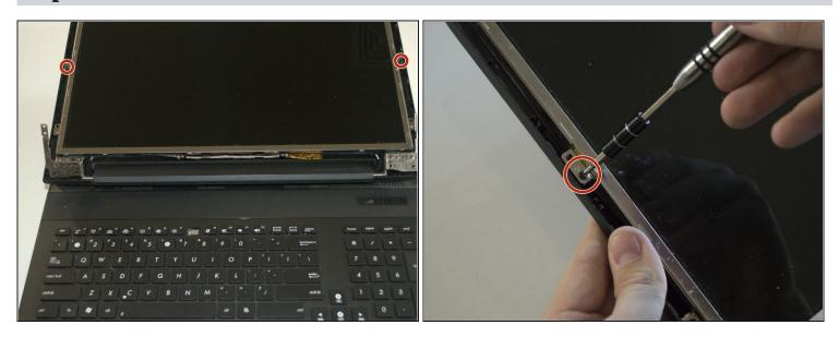
Remove the two 6mm Phillips #0 screws on either side of the screen using a Phillips #0 screwdriver.
