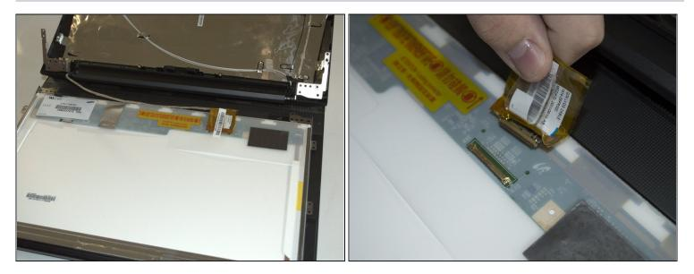
• Remove the screen from the laptop casing and flip it over. Peel the sticker above the connector back and firmly pull the connector out.
