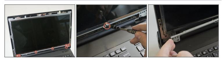
• Repeat the last step with the bottom bracket, removing eight 6 mm Phillips #0 screws using a Phillips #0 screwdriver. Set the bracket aside.
