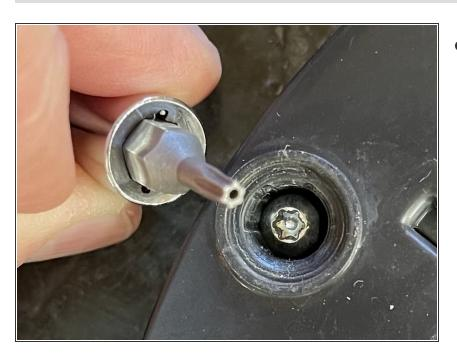
Also the front two screws are safety screws: they have a 6 sided star shape with a raised dimple in the center to prevent homebodies from casually opening the machine. (probably from the Sunbeam's (owns Mr. Coffee) legal dept.)
