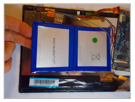
Peel the battery from the front panel.
