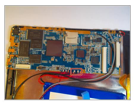
Melt the solder on the red and black wires and remove wires.
