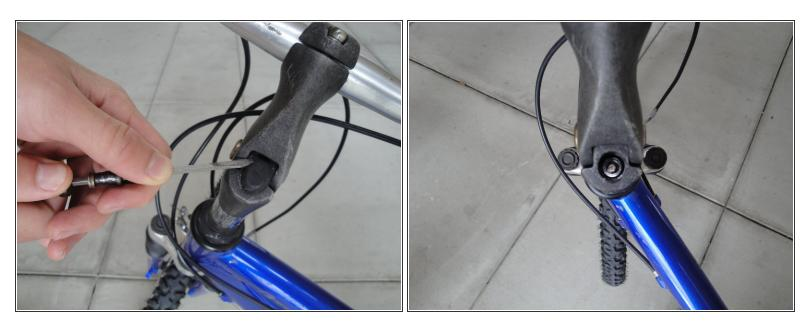
Remove the bolt cover with a flathead screwdriver.
