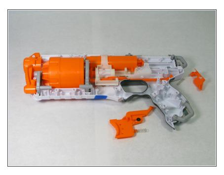
From the base, lift the action and the trigger.
