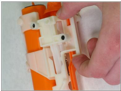
Screw the cover back onto the cylinder rotator.
