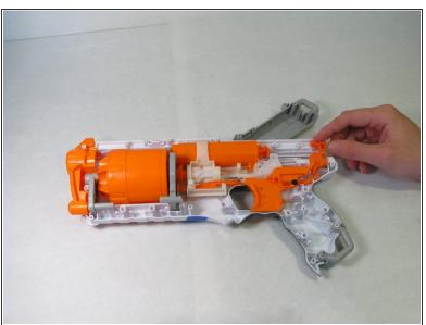
Screw the trigger and the action back in. Swing the gray gun charging slide out when putting the action back in.
