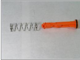
Turn the spring counter-clockwise to free the spring. Be careful at the beginning and the end of the process.
