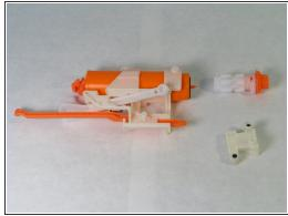
Unscrew screws (2) from the cylinder rotator mechanism.
