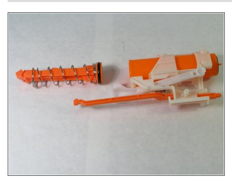
Remove the air plunger and the spring from inside the chamber.
