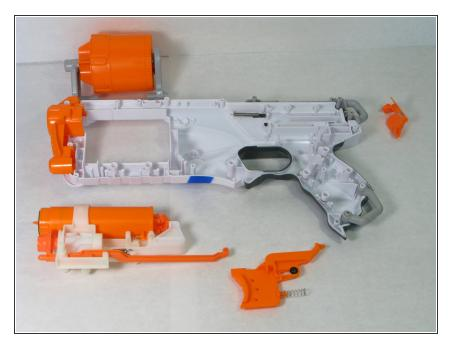
Lift the Nerf dart cylinder and the firing mechanism (spring chamber).
