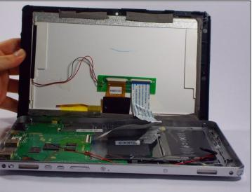
• Use the opening tool to pry the screen from the case applying pressure at each of the four corners of the screen.
