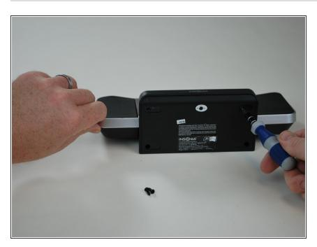
Begin unscrewing the six 11mm screws with a Phillips head screw driver.
