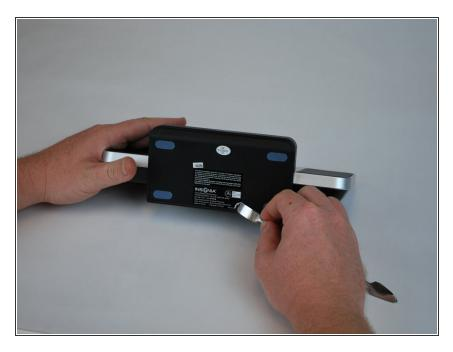
Begin by using the Metal Spudger to peel back the adhesive sticker and locate the screw beneath the sticker.
