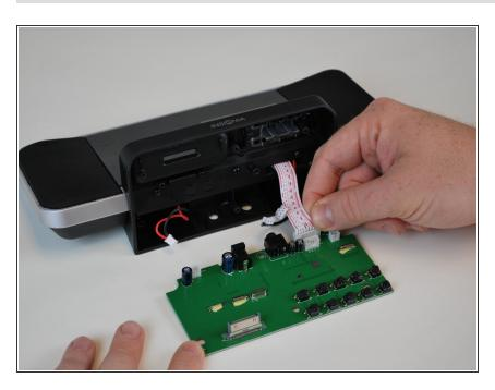
Remove the LCD screen plug. Then, follow the previous instructions in reverse, replacing the old motherboard with the new one to fix the 30-Pin Connector.
