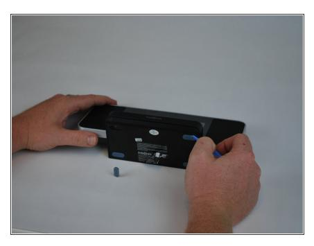
Continue peeling the rest of the gel stoppers from the bottom of the device.
