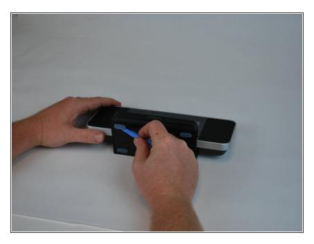
Using the Plastic Spudger, peel off the adhesive gel stoppers.
