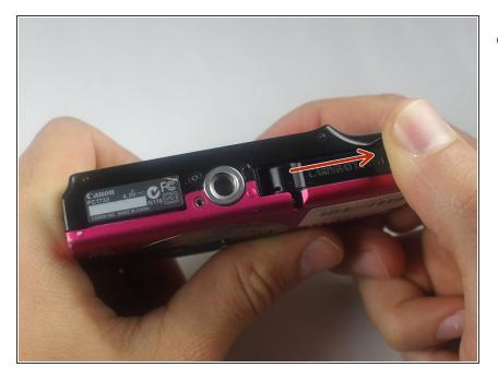
Open the Card/Battery latch by sliding the cover away from the camera in the direction indicated by the arrow.
