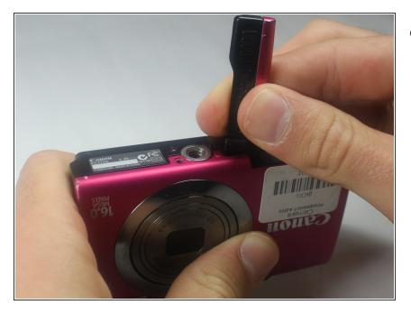
Gently rotate latch 90 degrees either clockwise or counterclockwise then remove it.
