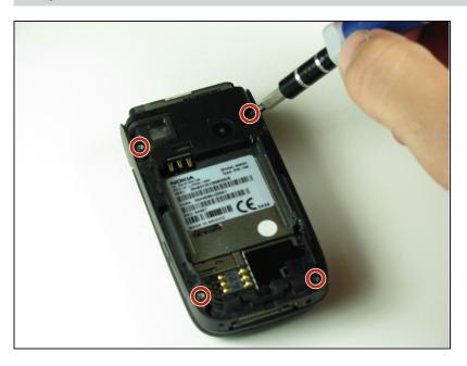
Use a T6 Torx screwdriver to remove the four 7.6 mm screws at the corners of the battery compartment.
