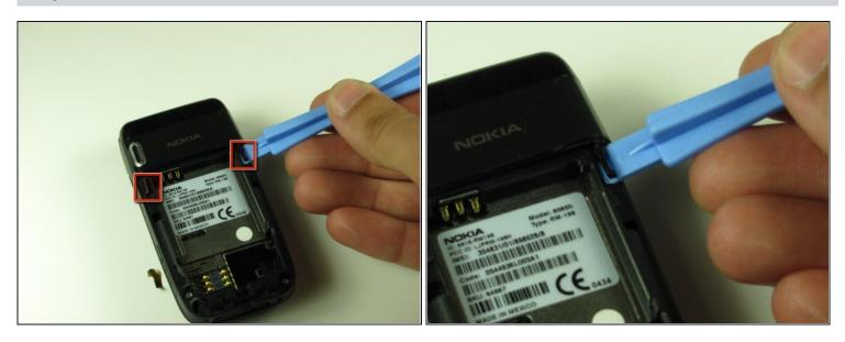
• Use the iFixit opening tool to pry out the two tabs at the top corners of the battery compartment.
