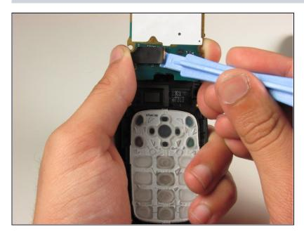
Find the underside of the motherboard and locate the ribbon cable that attaches the board to the rest of the phone. Use the plastic opening tool to slowly detach the ribbon cable connector, then pull the motherboard away from the frame.
