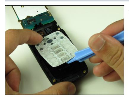
Pry the keypad out with the plastic opening tool once the motherboard is moved out of the way.
