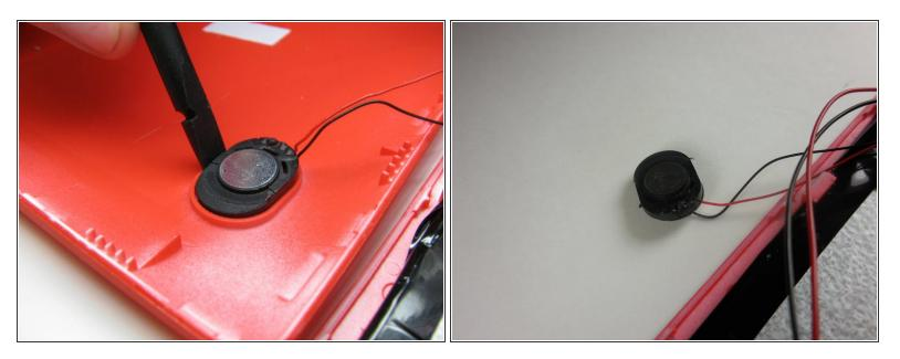
• After successfully separating the casing insert a plastic spudger between the case and the speaker. Carefully pry the speaker out. Once the speaker is removed set the back casing aside.
