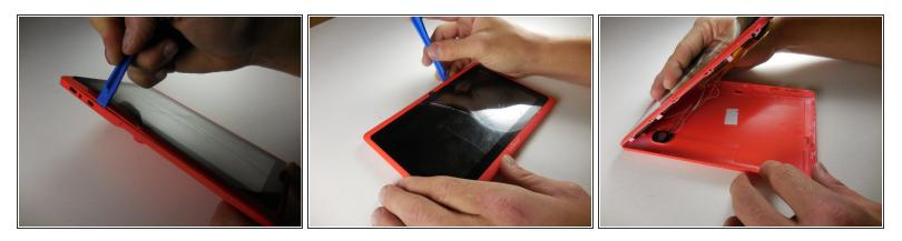
Insert the blue plastic opening tool where the case has a seam. Move side to side until you hear a clip pop. Move around the edge of the case until all clips are separated. The clips are 1.5 in. apart within the case.
