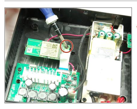
Unscrew the 10 mm screw holding the wireless audio module.
