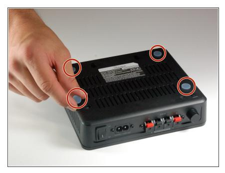
Remove the 4 rubber tabs on the bottom side of the receiver.
