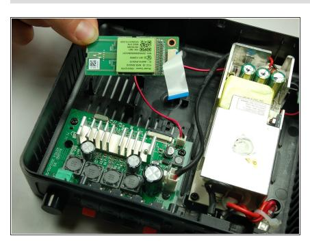
Using your fingers, slide the ribbon cable out from the under the black retaining flap to completely disconnect it from the device. To install the new wireless audio module chip, follow these instructions in reverse order.
