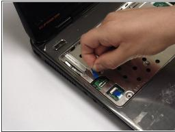
• Locate the palm rest cables. Lift the black levers and unplug the blue cables.
