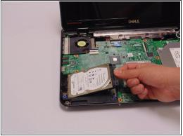
Lift and remove the hard drive.
