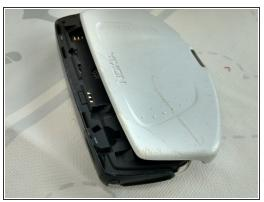
To take off the housing you need to turn the device upside down and push the release button down at the bottom of the phone and pull the cover down with your thumbs until you hear a click, and the cover should come free
