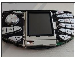
With the housing unclipped you should be able to lift it off.
