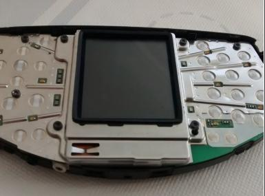
• Lift off the buttons to reveal a bare contact pad. Now you have removed the housing!
