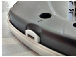
To take off the front bezel you need to put your nails under the clips pictured and pry off the case
