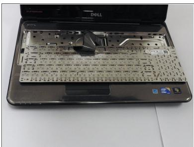
Carefully pull and turn the keyboard over.
