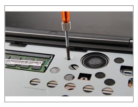
Remove the two screws securing the midframe.
