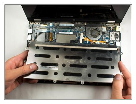
Now that the battery is disconnected from the device, lift the battery and gently remove it from the device. To reassemble your device, follow these instructions in reverse order.
