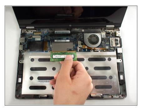
Grab the RAM module and carefully pull it out from its position.
