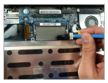
Use a plastic opening tool to disconnect the battery connector from the motherboard.
