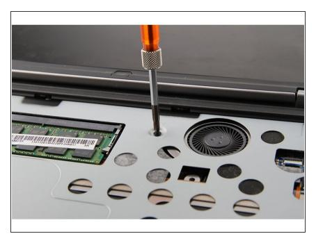
Remove the two screws securing the midframe.
