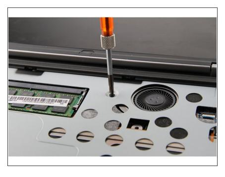
Remove the two screws securing the midframe.
