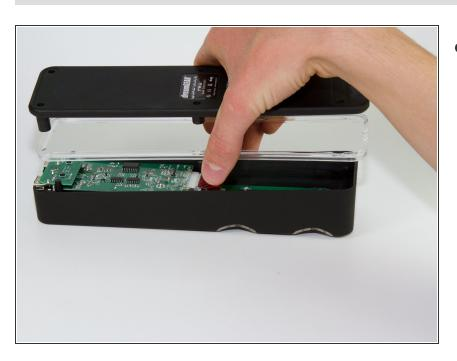
Gently remove the bottom of the device.
