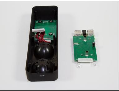
• Use a plastic opening tool or similar tool to gently pry the power ribbon cord out of its port.
