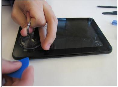
Use the suction cup and lever tool tool to pry the front screen from the tablet.
