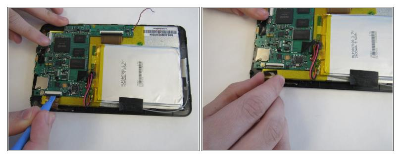
Pull up the switch to remove the input connector.
