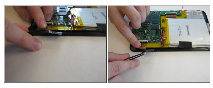
Using the tweezers, remove the black tape connecting the screen to the motherboard.
