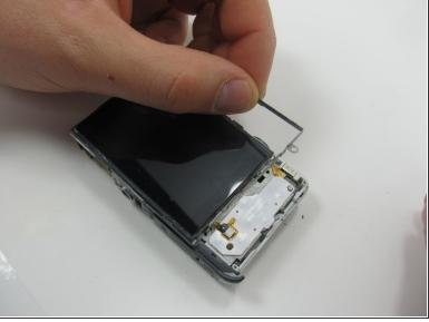
Remove the 3.1mm screw on the top-right side of the LCD display screen.
