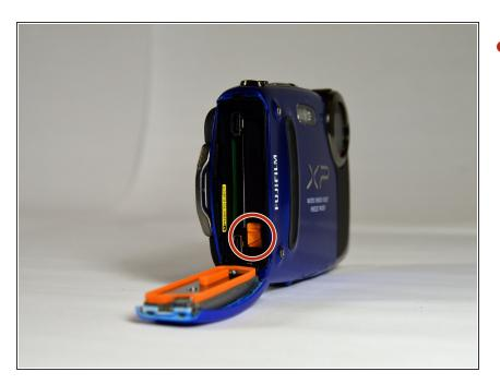
Slide small orange tab to release the battery.
