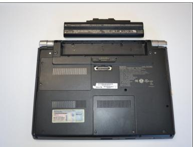
• Use a fingernail or plastic opening tool lift the battery while holding the release latch. Rotate the battery up and away from you to remove it from the laptop.
