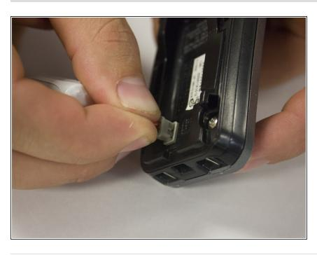
Take the replacement battery and push the grey connector back into the phone.
