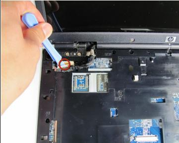
Use the plastic prying tool to disconnect the screen cable from the system board.
