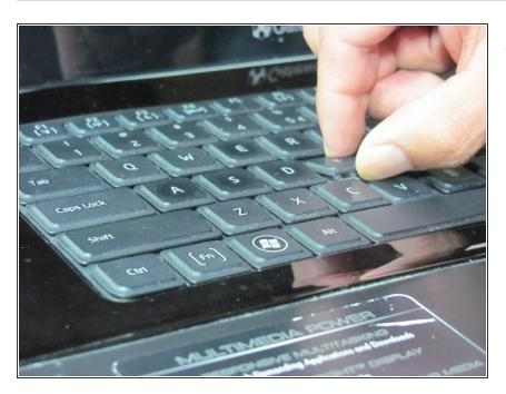
Using your fingernail, apply pressure upward from underneath the key to pry it loose from its bearings.
