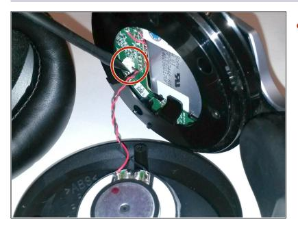
Using tweezers, gently pry the red and black speaker wires from the attached socket.
