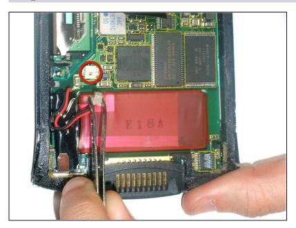
Using the <u>tweezers</u>, carefully disconnect the battery cable from the port
