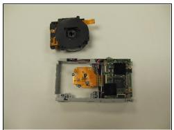
• The optic assembly should now be free. Use a pry tool to lift it far enough up that you can grab and remove it.
