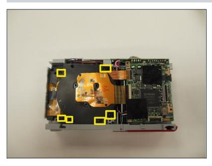
Remove the six 3.25 mm screws securing the optic lens to the camera frame.
