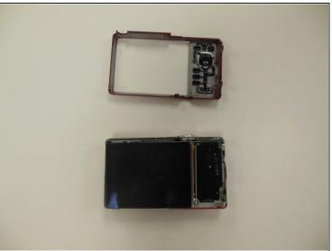
Using both hands, carefully pull the frame apart from the camera.
