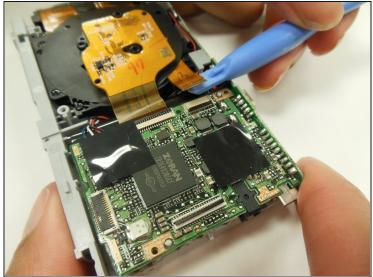
• There is a small ribbon attaching the optical lens piece to the motherboard. Using a plastic opening tool, gently lift up on this ribbon's clamp, detaching it from the motherboard.
