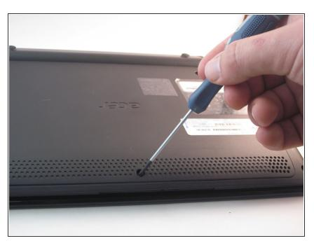
Locate the 4 mm Phillips #1 screw at the bottom of the back panel. Using the Phillips head screwdriver, remove the screw. Place the screw somewhere it will not be lost. Then remove the back panel by gently sliding it towards the front.
