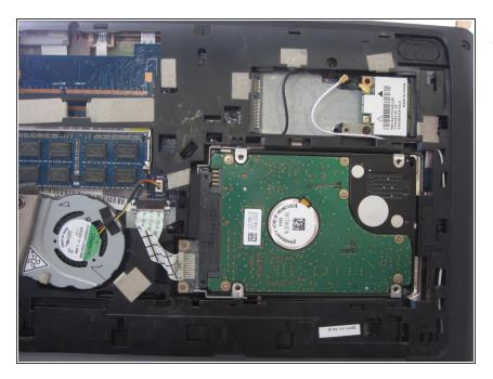
After removing the back panel, locate the hard drive.
