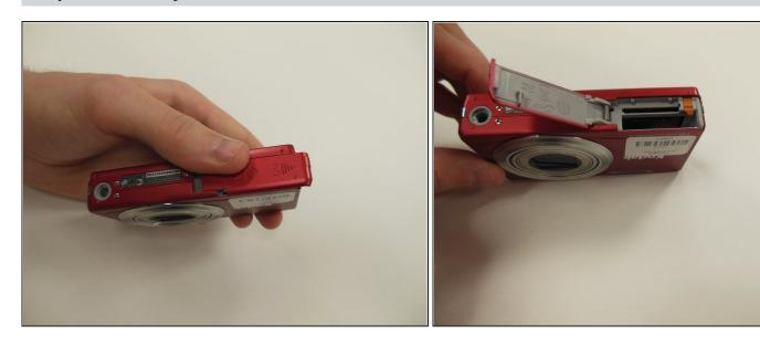
First, press in and slide forward the battery latch as indicated by the arrow.
