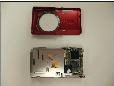
Carefully lift and remove front covered panel from the camera.
