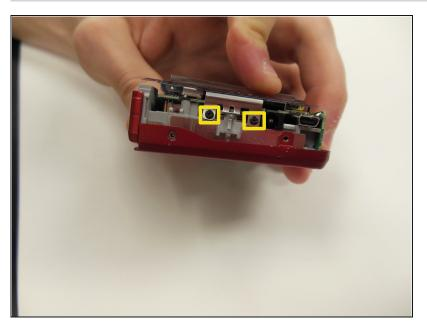
On the right side of the camera, locate and remove the two 3.25 mm screws as highlighted.
