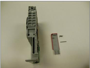
The latch can now easily be pulled out of place and removed.
