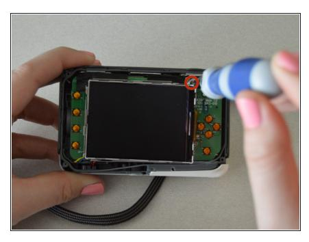
Remove screw connecting the top right of the screen to the mother board.
