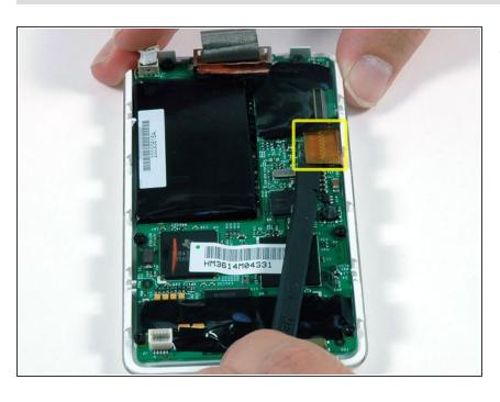
Use a spudger to carefully disconnect the orange touch wheel cable from the logic board.
