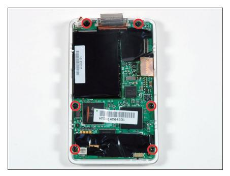
Remove the 6 black T6 Torx screws securing the logic board to the front panel.
