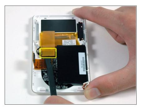
Use a spudger to carefully disconnect the orange display ribbon from the front panel.
