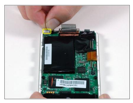
Carefully disconnect the white battery connector from the logic board. Be sure to pull only on the connector itself and not on the cables.
