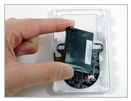
• Lift the battery out of the iPod.
